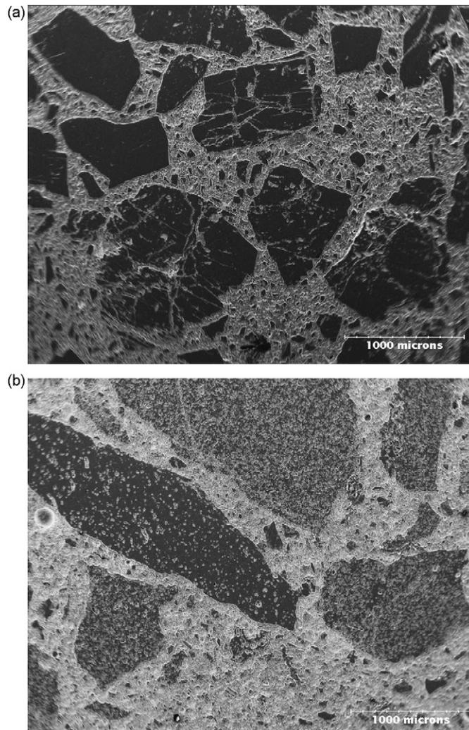
Fig. 1. Microstructure of studied refractories: (a) And-LCC; (b) Bau-ULCC.
