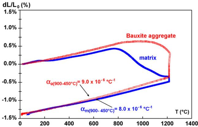
Fig. 9. Thermal expansion behaviours obtained on the bauxite aggregates and the matrix of Bau-ULCC castable.
