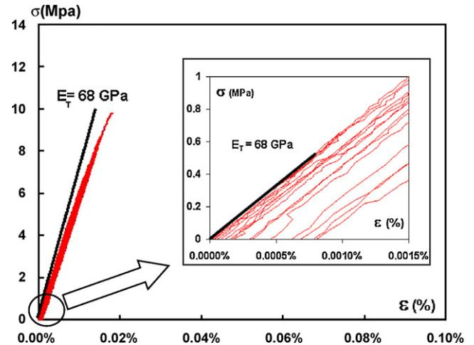
Fig. 4. Stress–strain tensile curves of And-LCC at room temperature after treatment at  $110^\circ\text{C}$ . Zoom of the initial part of the curves that illustrates the early determination of the Young's modulus  $E_T$ .
