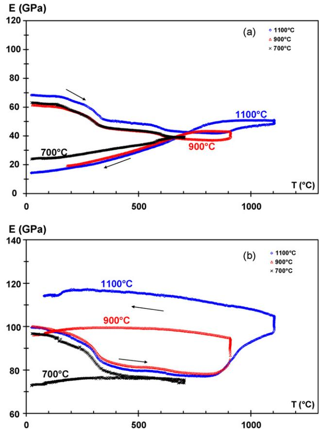
Fig. 6. Evolution of the Young's modulus measured by the ultrasonic technique ( $E_{us}$ ) for both castables during different first thermal cycles: (a) And-LCC; (b) Bau-ULCC.
