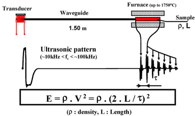
Fig. 2. Experimental set-up used for Young's modulus measurement at high temperature by long bar mode ultrasonic pulse technique.
