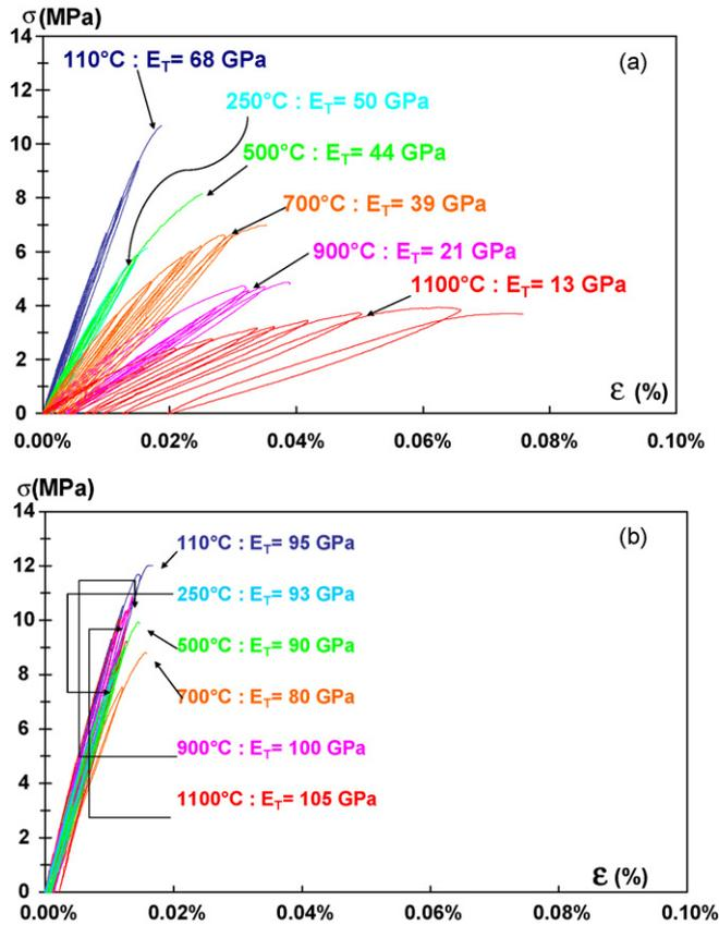
Fig. 8. Tensile behaviour at room temperature of both castables treated at different temperatures: (a) And-LCC; (b) Bau-ULCC.
