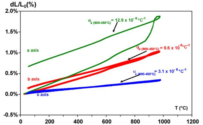
Fig. 11. Comparison of the dilatometric behaviour in the three directions of an andalusite single crystal with the matrix of the And-LCC castable.
