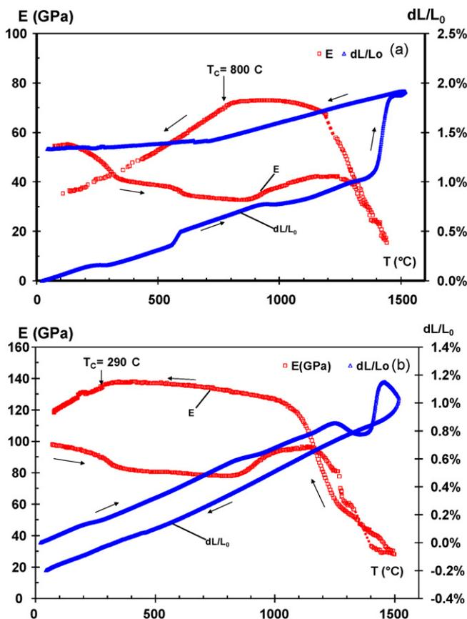
Fig. 5. Variation of the Young's modulus measured by the ultrasonic technique ( $E_{us}$ ) and thermal expansion for the two castables: (a) And-LCC; (b) Bau-ULCC.
