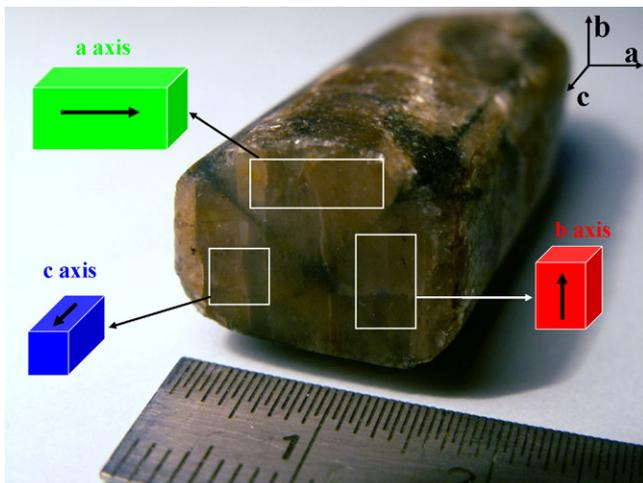
Fig. 10. Scheme of the dilatometric sample extraction procedure applied on an andalusite single crystal to investigate its thermal expansion anisotropy.
