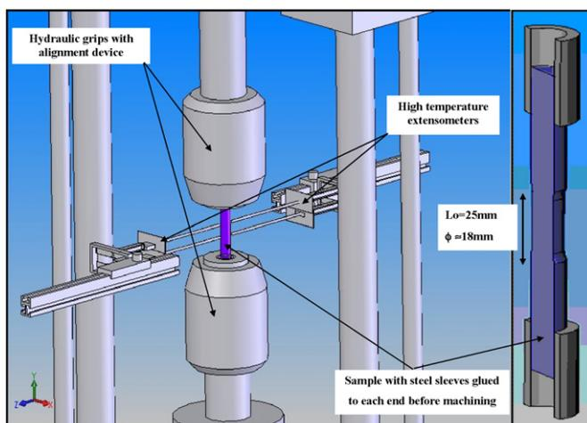
Fig. 3. Scheme of the tensile test device.
