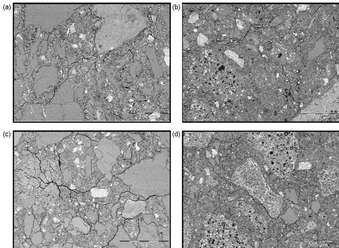
Fig. 7. Identification of damage in the two castables after thermal treatments: (a) And-LCC at 700 °C; (b) Bau-ULCC at 700 °C; (c) And-LCC at 900 °C; (d) Bau-ULCC at 900 °C.
